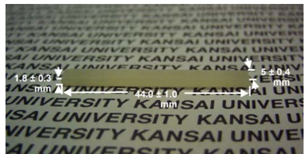
Figure 1 Photograph of the composite specimen prepared from solution AC1 and post-dried at 70°C.
